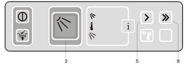
The machine is pre-set to slow-speed transport: Button 5 blinks.
