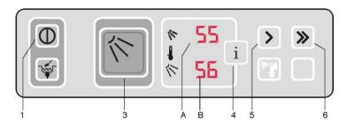
> Press the on/off button (1) to switch on the machine.
