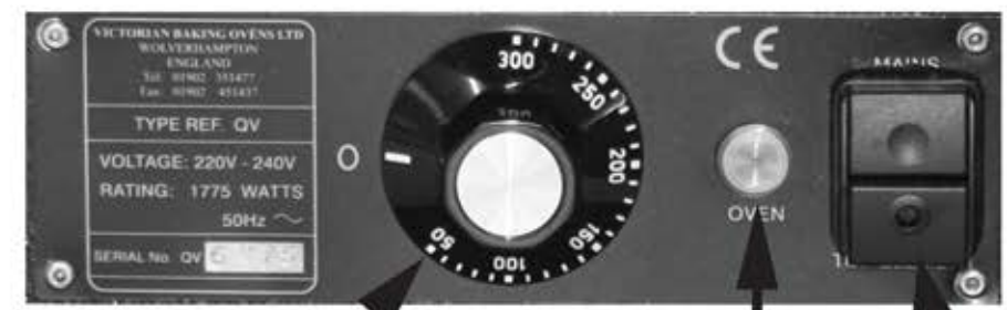
thermostat control knob CONTROL PANEL green neon oven indicator on/off switch
