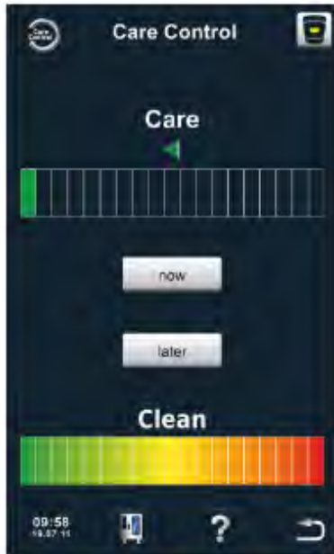
Automatic display of cleaning request as soon as CleanJet® +care cleaning is necessary.
