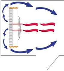
In the unlikely event that your blast chiller is taking longer to perform its chilling cycle, ensure that the system is operating in the correct way. A possible explanation is that the fan system has been installed the wrong way round. As a result the airflow within the blast chiller will not work as effectively as it should. See the diagram.
