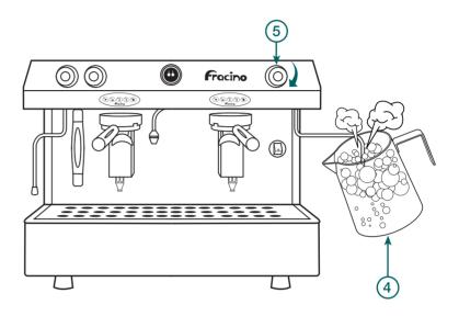
**4)** When the 'tone' changes it is an indication that the milk is about to boil. Alternatively you can use a jug thermometer and heat to the required temperature of 70-75°C **5)** At this point turn off the steam. DO NOT ALLOW THE MILK TO BOIL AS IT WILL GO FLAT. The milk should have risen to almost fill the jug and be of a creamy/foamy consistency.
