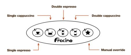
**Single espresso:** use the single filter holder, one shot of coffee, one espresso cup and press the single espresso button.
