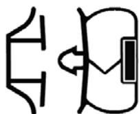
Damaged gaskets are easily replaced. Simply pull out existing part and push new gasket into channel (gasket retainer) at centre and work along, pushing gasket into channel.
